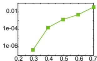
[Convergence of  $E_{\text{total}}$  versus `wvl_hgrid` for a silane]
