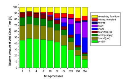
Figure 53: Relative amount of wall clock time for the most costly code sections.
