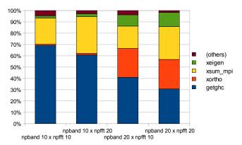
Figure 23: CPU time distribution for the ABINIT parallel eigensolver (standard test case: 107 gold atoms) with respect to the number of "band" cores (npband) and "FFT" cores (npfft).
