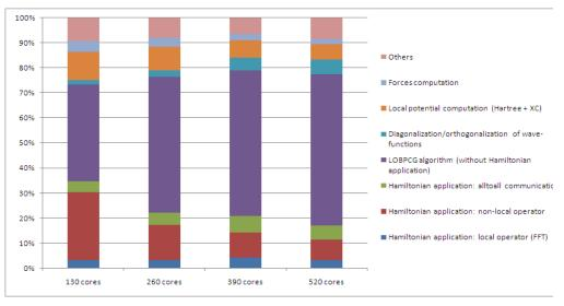
Figure 24: Repartition of CPU time in ABINIT routines varying the number of CPU cores.
