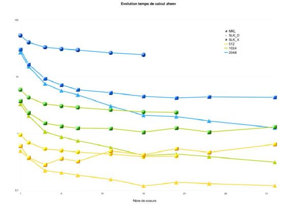
Figure 22: CPU time (sec.) per process needed by a single call to ZHEEV *ScaLAPACK* routine with respect to number of MPI process for several sizes of square matrix (512, 1024, 2048) and several *ScaLAPACK* implementations
